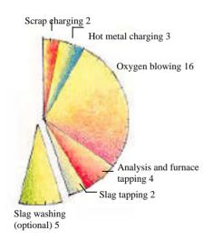
*Figure 6 A typical BOS production cycle. The complete cycle of production required to produce 280 tonnes of molten steel is about 27 minutes*
