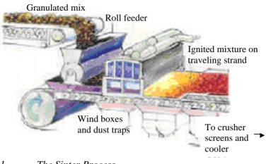
Figure 1 The Sinter Process
