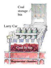
Figure 2 Coke Oven Batteries have up to 100 narrow ovens with heating chambers between each oven
