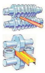
Figure 12. Top: Typica/2-high merchant strand. Bottom: Arrangement of rolls in a universal beam mill, rolling all four sides of the beam in a single pass.
