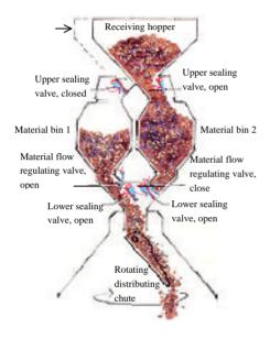
*Figure 5* The Paul Wurth top provides highly efficient distribution of raw material feed
