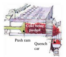
*Figure 3 Heating for about 18 hours distils volatiles from coal to produce coke*
