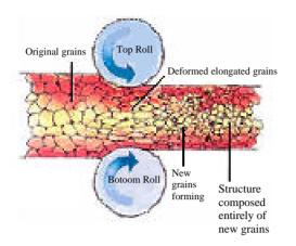
Figure 10. Deformation of steel grain structure under rolling, and development of a new grain structure.
