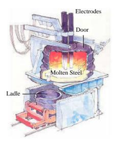
Fig 8 Electric Arc Furnace
