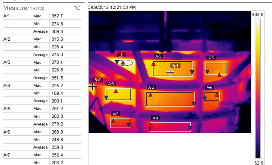
Figure 7: FLIR E60 Thermovision of Balcony Region with Wear Lining at 1300 heats
