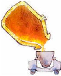
Secondary steelmaking or ladle refining (e.g. vacuum treatment, inert gas stirring, ladle furnace metallurgy) occurs in the ladle after molten steel has been tapped from the steelmaking vessel. The purpose is to increase furnace productivity by performing some of the operations normally done in the steelmaking vessel. It also improves steel quality.
